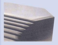
The magnetic core of the transformers is built up of cold rolled grain oriented magnetic steel laminations. The special cutting and stacking methods result in low no load losses and noise levels. Core leg and yoke laminations are interleaved in mitered joints in order to facilitate the passage of the magnetic flux and to avoid hot spots and reduce no load losses, no load current and low noise level.
