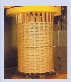
The windings are designed to optimize dynamic, thermal, mechanical & electrical stresses depending upon the current & voltage requirements, spiral, cross over helical, continuous disc, partly interleaved or fully interleaved windings are used depending on the specific design criteria.
